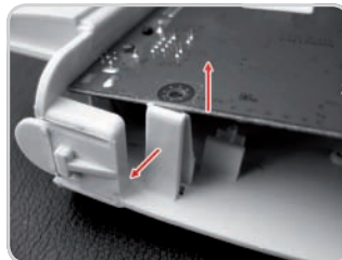
Release the front position.
